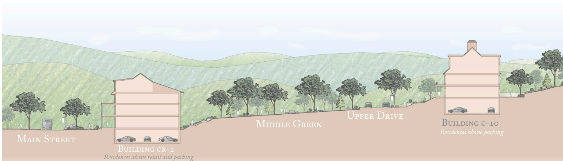
SECTION THROUGH MAIN STREET AND MIDDLE GREEN demonstrates how buildings and roadways are layered with the landscape to complement the existing grade. Buildings along Upper Drive are elevated above the roadway with terraces, steps and stone walls.
